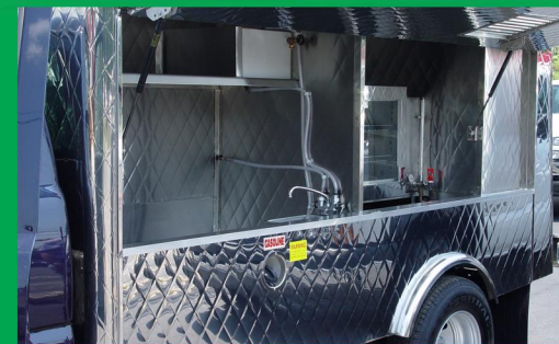
Three comp + hand sink and large capacity coffee/hot water
